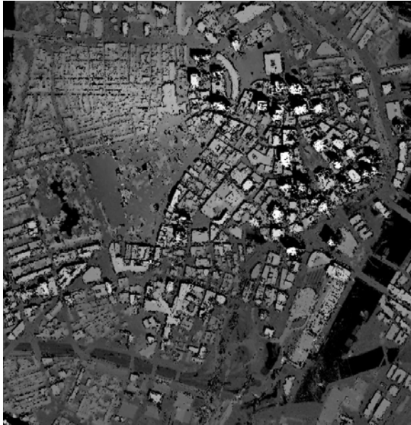
Figure 12: The final DEM computed by fusing all DEMs generated from the set of nine Ikonos images. The elevations are encoded in greyscale such that lower elevations are dark and higher elevations are light. Unreliable elevations are encoded in black.
